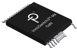
InSOP-24D (C-Package) MSL-3 Rated - wave solder and reflow
